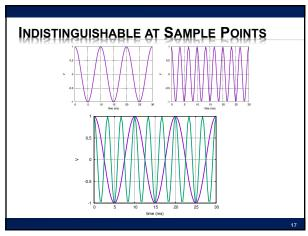
Observe: we must, at least, sample at twice the frequency of the signal we are trying to capture
