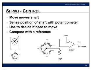
SERVO - CONTROL x Compare with a reference Assume comparator computes: Vout=A\*(V+ - V.) Vout =  $A^*(V_{control} - V_{potentiometer})$ What is Vout when  $V_{potentiometer} < V_{control}$ ? What is Vout when Vpotentiometer>Vcontrol? To Motor
