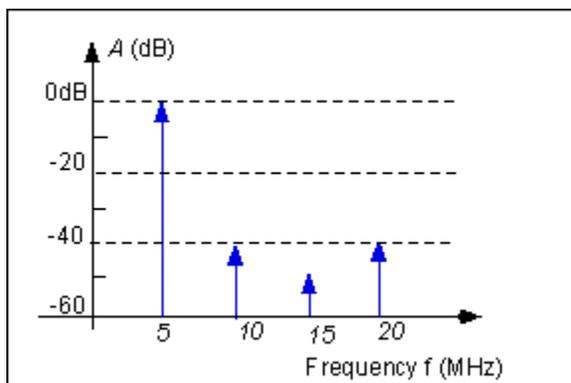
Figure 6: Spectrum of a distorted sinusoidal signal of 5 kHz.
