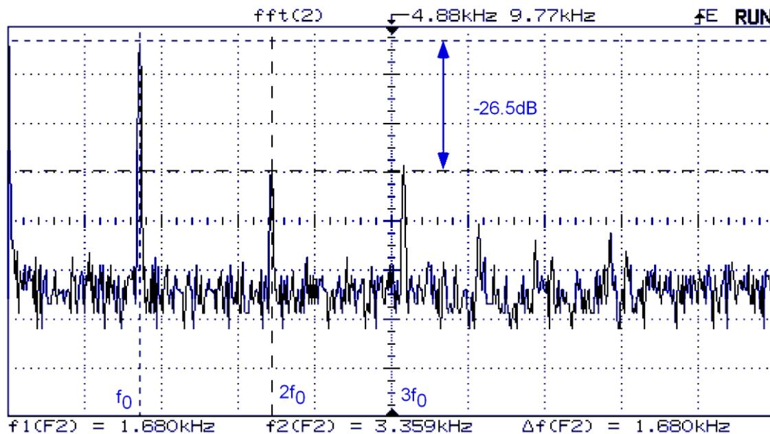
Figure 3: Spectrum of a distorted sinusoid with fundamental frequency  $f_0=1.68\text{kHz}$ .
