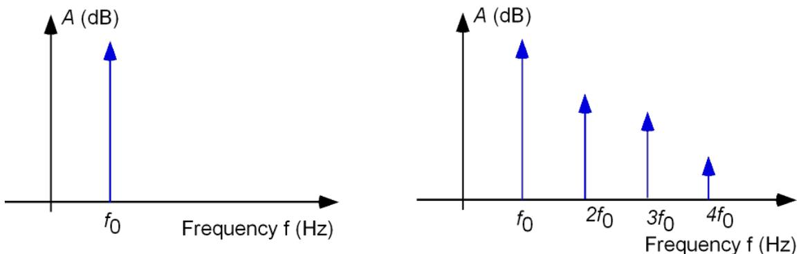
Figure 2: Spectrum of (a) a pure sinusoid and (b) a distorted sinusoid.
