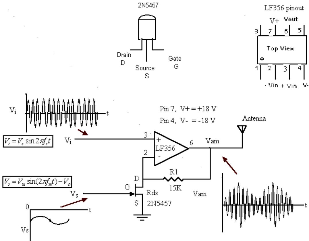
Figure 4: A Simple AM Modulation/Transmitter Circuit
