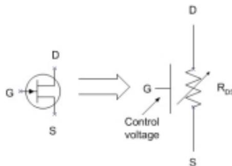
Figure 5: A JFET used as a voltage-controlled resistor.
