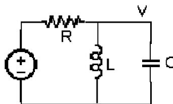
Figure 3: LC circuit.
