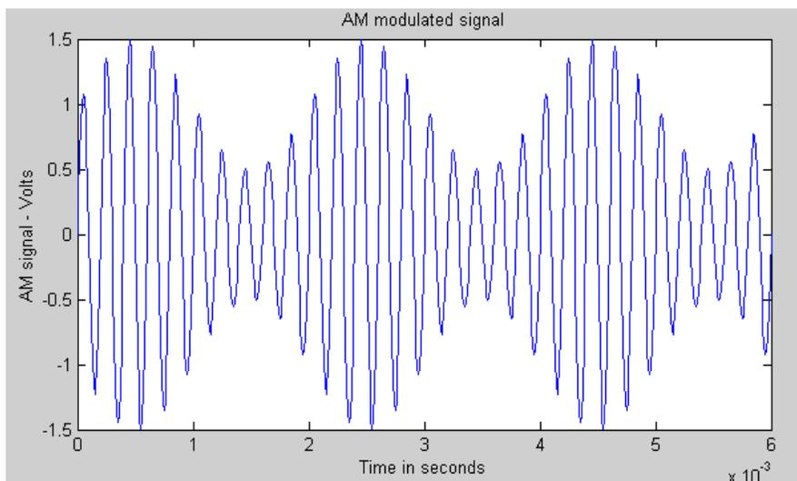
Figure 1: Am Modulated Signal ( $f_m=500$  Hz and  $f_c=5$ kHz)
