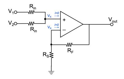
Both opamp inputs are at the same voltage, which is labeled  $V_X$  here, and the current into both inputs is 0. We can do KCL at both inputs:
