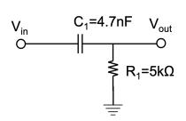
High pass filter.  $f_C = \frac{1}{2\pi RC} = \frac{1}{2\pi \cdot 5k\Omega \cdot 4.7nF} = 6.77 kHz$
