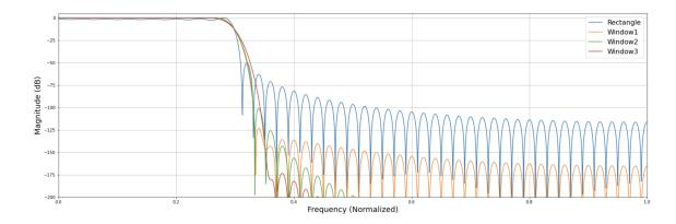
The LPF filter frequency response from using a rectangular window is labeled, and the other three filters are from applying 3 different windows to the sinc function: Blackman, Hamming, and Hann. All filters and windows are the same length. The frequency response of the four windows functions are given below. Note the different scales on the y-axis.
