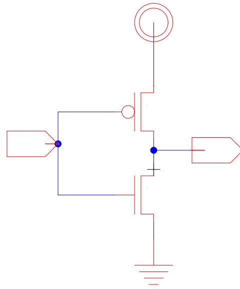
1. What current flows in the inverter in steady state? Think about the region of operation of the devices for each input case.
