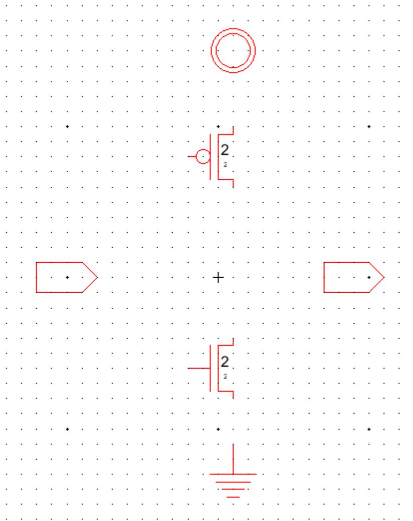
To draw wires between components, hover over a node until the component is highlighted and the node is marked with a cross. Use your left mouse button to select the component and node.
