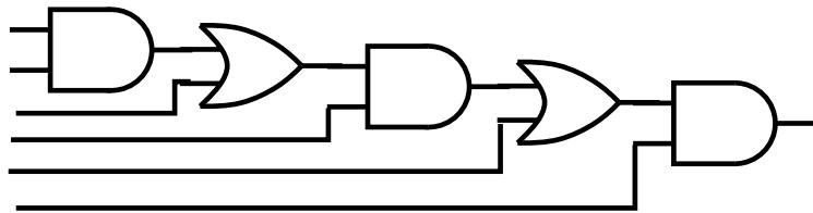
Assume  $R_{drive} = \frac{R_0}{2}$  sizing of gates from previous page, and input also driven by  $R_{drive} = \frac{R_0}{2}$ . Assume each implementation has an output load of  $2C_0$ .
