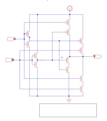
3. Assuming this circuit is loaded by an inverter (equivalently, the inverter input of another copy of this circuit), what is equivalent RC circuit on the output if A=1?  $(C_{diff} > 0)$
