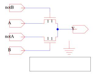
(ground terminal just used for NMOS body contacts)
