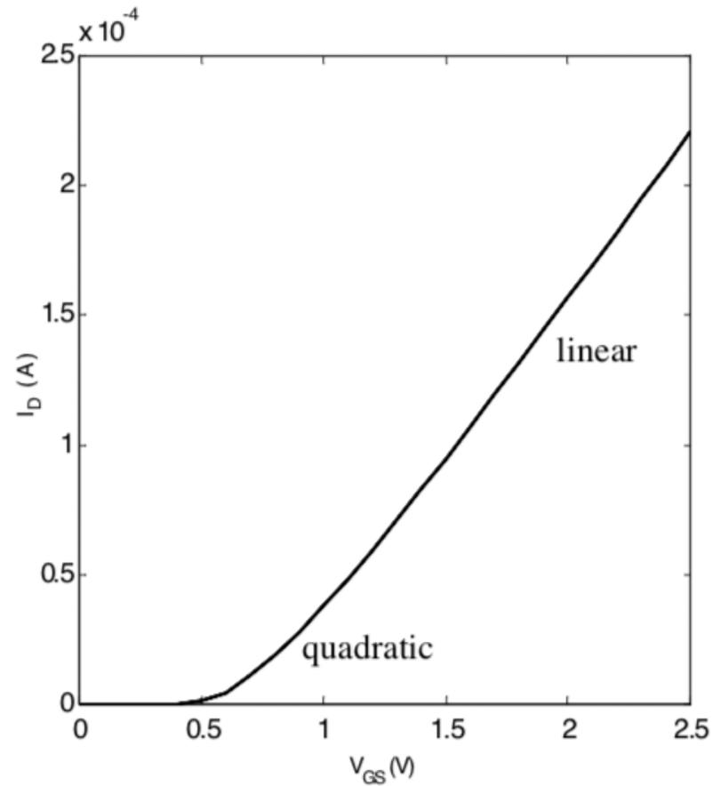
(b) Short-channel device ( $L_d = 0.25 \mu\text{m}$ )
