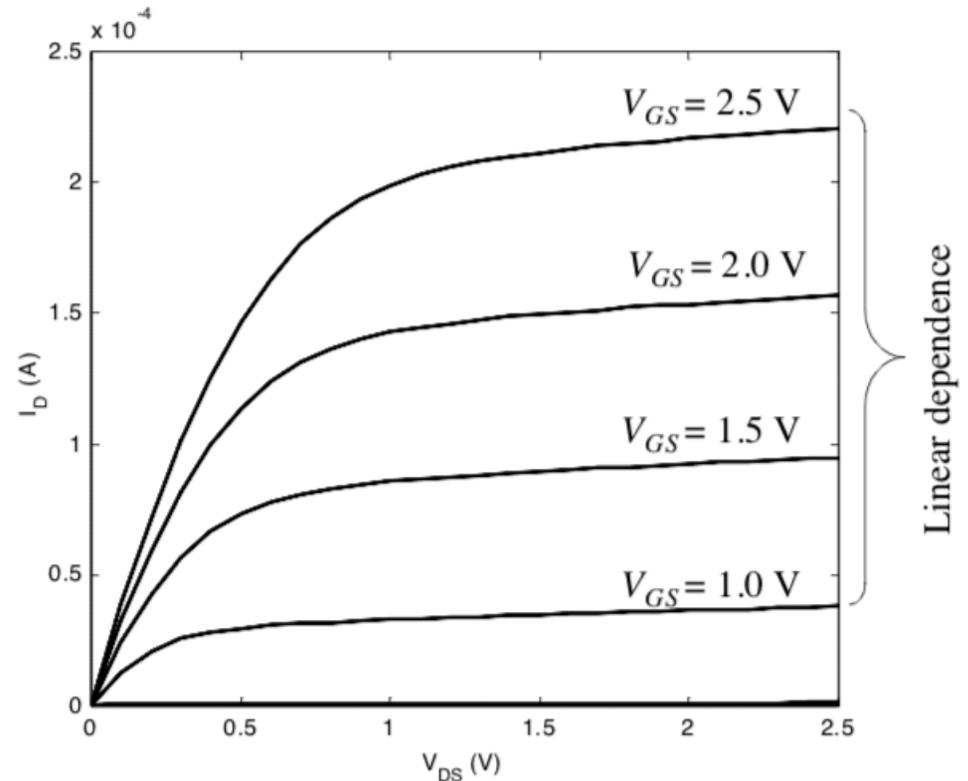
(b) Short-channel transistor ( $L_d = 0.25 \mu\text{m}$ )
