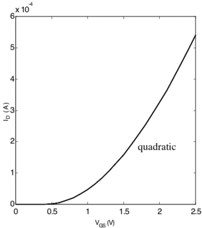
(a) Long-channel device ( $L_d = 10 \mu\text{m}$ )
