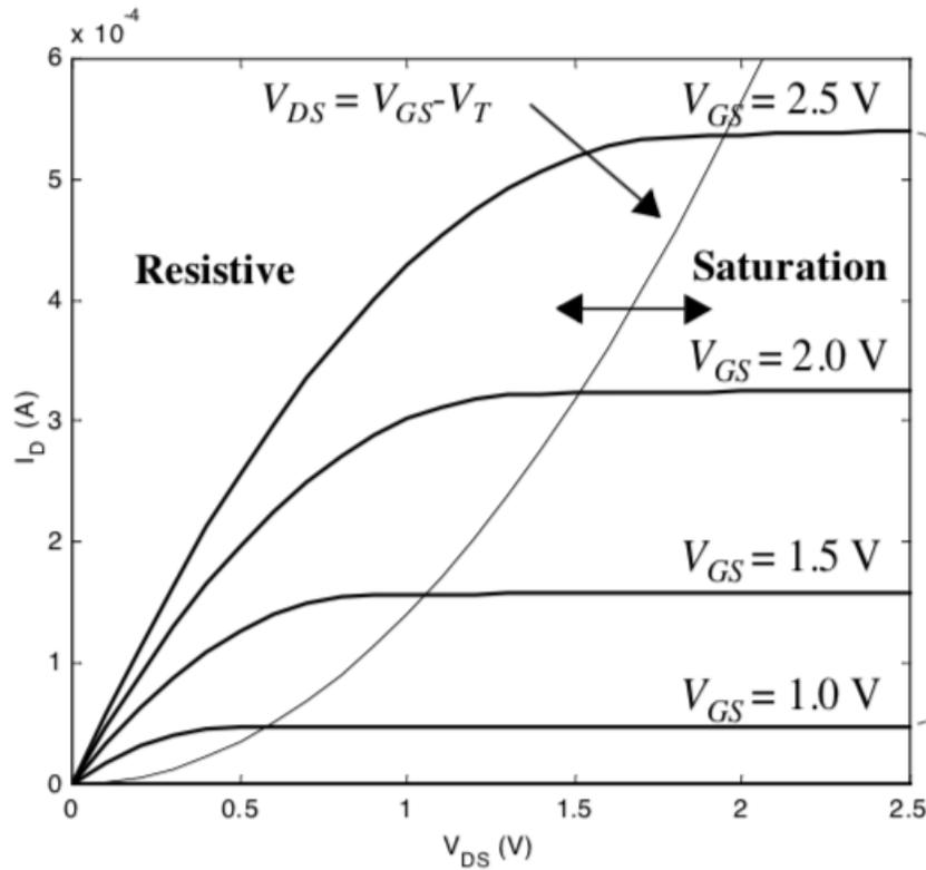
(a) Long-channel transistor ( $L_d = 10 \mu\text{m}$ )
