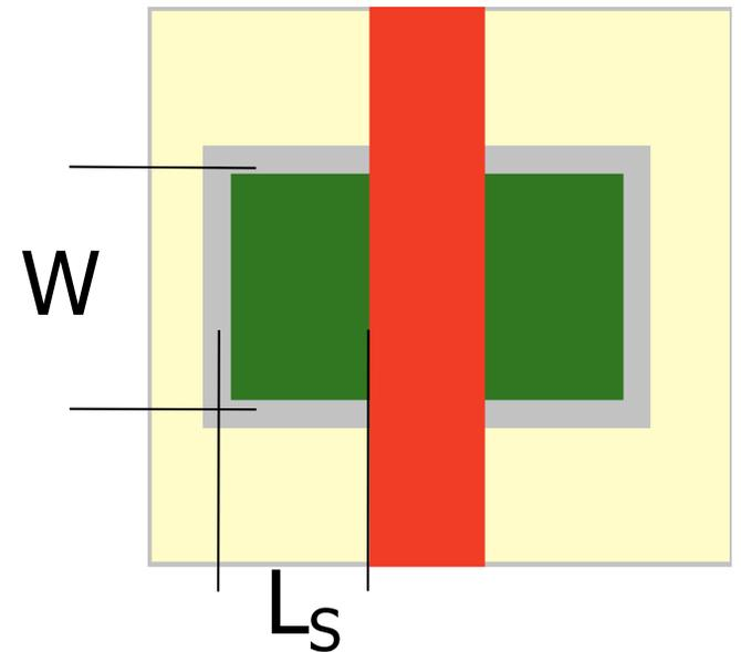
$$C_{diff} = C_j L_S W + C_{jsw} (2L_S + W)$$
