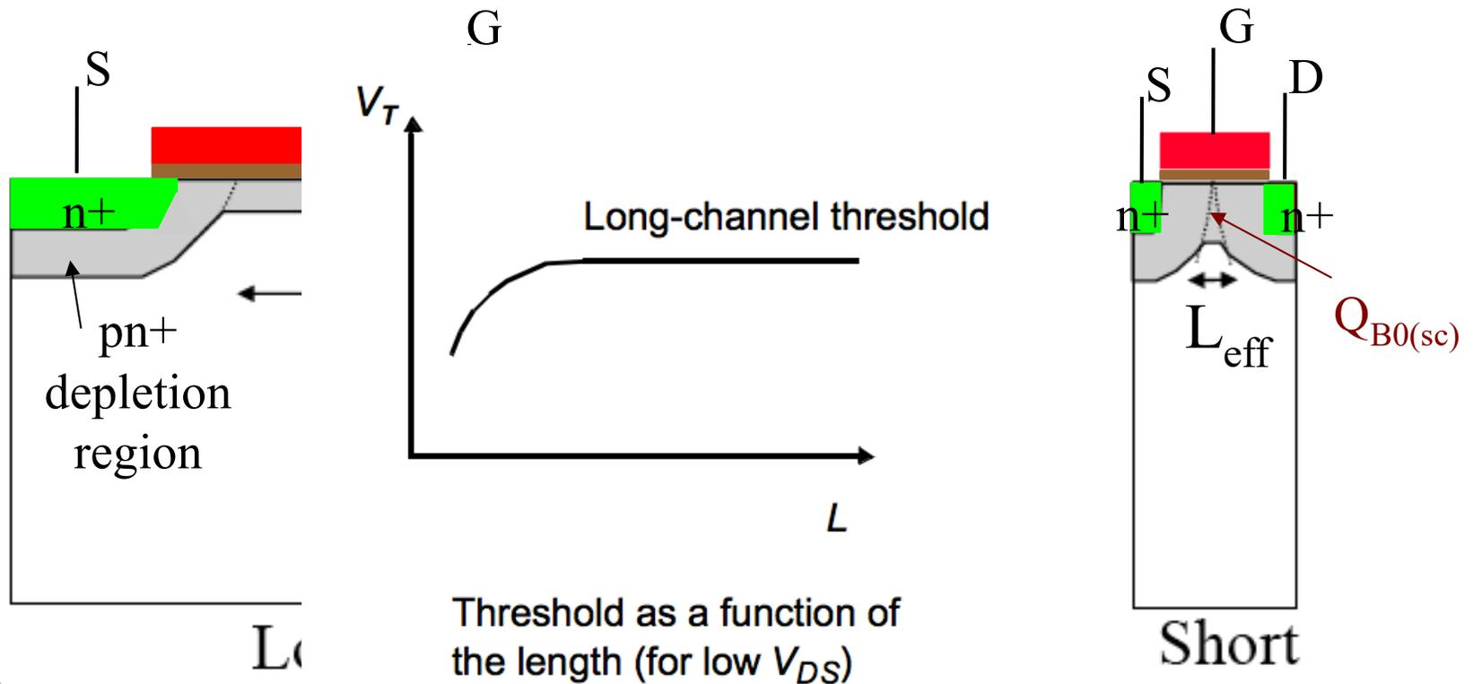
$$V_{T0} \text{ (short channel)} = V_{T0} - \Delta V_{T0}$$
