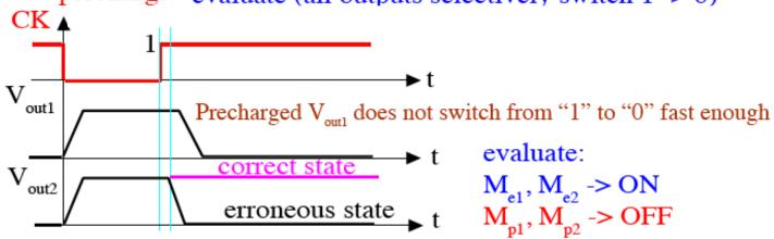
PROBLEM: ALL STAGES MUST EVALUATE SIMULTANEOUSLY SINGLE CLOCK DOES NOT PERMIT PIPELINING OF STAGES
