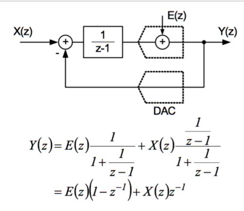
Output is equal to delayed input plus filtered quantization noise
