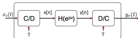
$$X(e^{j\omega}) = \frac{1}{T} \sum_{k=-\infty}^{\infty} X_c \left[ j \left( \frac{\omega}{T} - \frac{2\pi k}{T} \right) \right] \quad y_r(t) = \sum_{n=-\infty}^{\infty} y[n] \frac{\sin[\pi(t-nT)/T]}{\pi(t-nT)/T}$$
