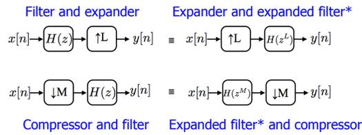
\*Expanded filter = expanded impulse response, compressed freq response
