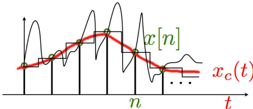
Multiple signals go through the samples, but only one is bandlimited within our sampling band
