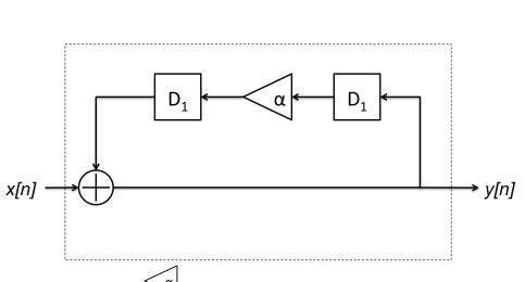
Above, the symbol  $\triangleleft \alpha$  denotes multiplication by a scalar  $\alpha$ : if the input is w[n], the output is  $\alpha w[n]$ . The symbol  $\square_1$  denotes a delay by one sample: if the input is w[n], the output is w[n-1].
