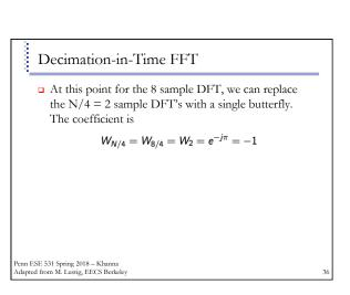
□ At this point for the 8 sample DFT, we can replace the N/4 = 2 sample DFT's with a single butterfly.
