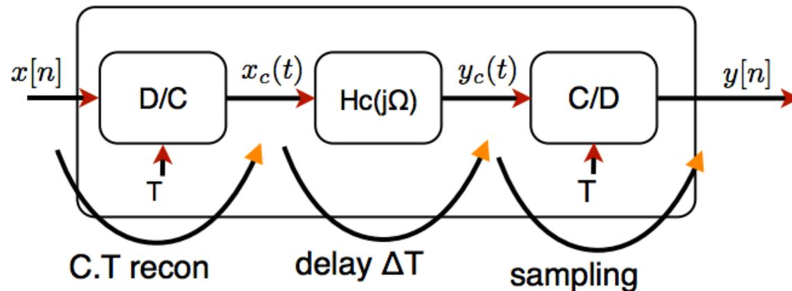
$$y[n] = y_c(nT) = x_c(nT - T \cdot \Delta) \quad x_c(t) = \sum_k x[k] \text{sinc}\left(\frac{t - kT}{T}\right)$$
