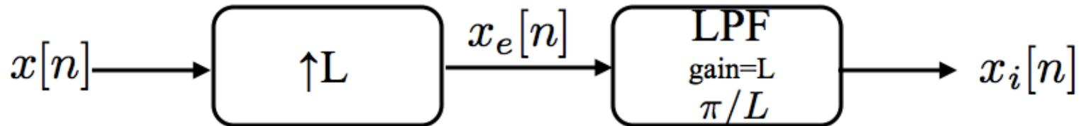
$$\begin{aligned} X_e(e^{j\omega}) &= \sum_{n=-\infty}^{\infty} \underbrace{x_e[n]}_{\neq 0 \text{ only for } n=mL \text{ (integer } m)} e^{-j\omega n} \\ &= \sum_{m=-\infty}^{\infty} \underbrace{x_e[mL]}_{=x[m]} e^{-j\omega mL} \end{aligned}$$
