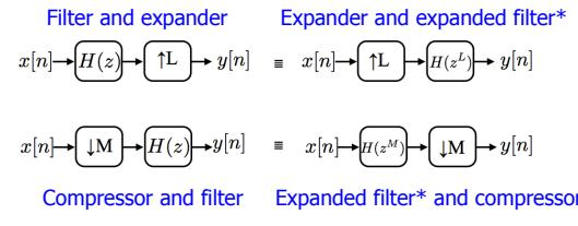
\*Expanded filter = expanded impulse response, compressed freq response
