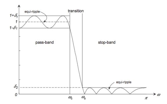
• For the low-pass filter shown above the specifications are
