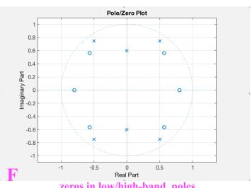
zeros in low/high-band, poles in mid-band -> Band stop filter
