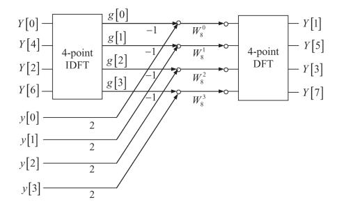
The diagram above shows 7 multipliers and 4 subtractors for a total cost of \$110.
