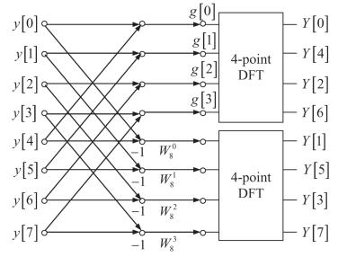
a) If Y[0] = Y[2] = Y[4] = Y[6] = 2, then the IDFT gives us g[0] = 2, g[1] = g[2] = g[3] = 0. We then can solve for y[4] = g[0] - y[0] = 2 - 1 = 1, and y[5] = y[6] = y[7] = 0.
