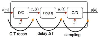
$$y[n] = y_c(nT) = x_c(nT - T \cdot \Delta) \quad x_c(t) = \sum_k x[k] \operatorname{sinc}\left(\frac{t - kT}{T}\right)$$
