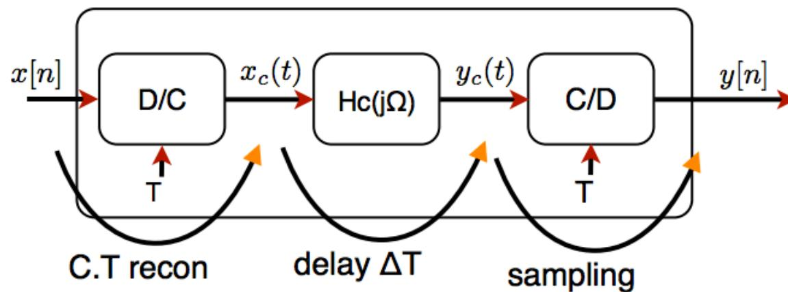
$$x_c(t) = \sum_k x[k] \text{sinc}\left(\frac{t - kT}{T}\right) \quad y_c(t) = x_c(t - T\Delta)$$
