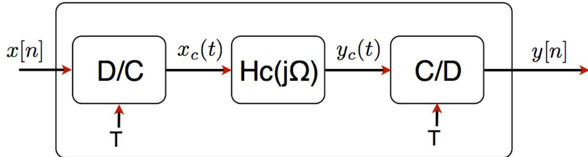
$$Y_c(j\Omega) = H_c(j\Omega)X_c(j\Omega) \quad Y(e^{j\omega}) = \frac{1}{T} Y_c(j\Omega) \Big|_{\Omega=\omega/T}$$
