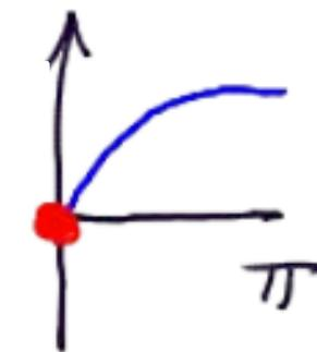
$$H(e^{j\omega}) = j e^{-j\omega M/2} \left[ \sum_{k=1}^{(M+1)/2} d[k] \sin \left[ \omega \left( k - \frac{1}{2} \right) \right] \right]$$
