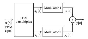
(a) The TDM input, w[n], is assumed to be the sequence of interleaved samples of two signals,  $x_1[n]$  and  $x_2[n]$ , such that
