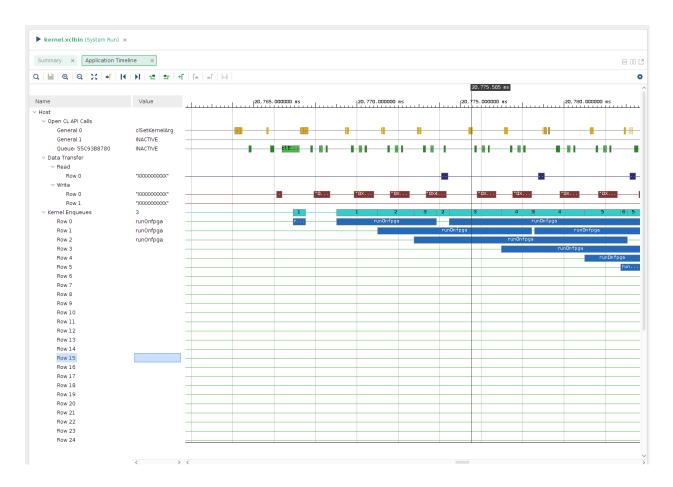
16. If you scroll forward in the timeline, you can see overlap between computation in the cpu and the fpga as shown below.
