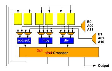
(d) What is the resource bound for this computation on a VLIW datapath with a single add/subtract unit, a single multiplier, and a single divider (as shown)?
