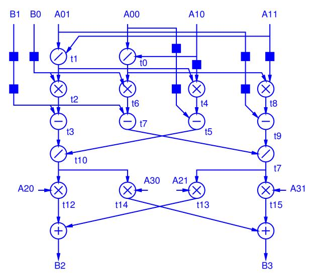
Note registers added (small squares) to balance path delays from inputs. As shown, assumes a register on the output of each operator.
