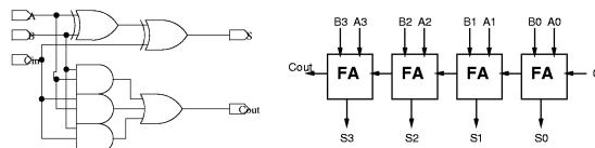
What is area and delay for N-bit RA adder?
