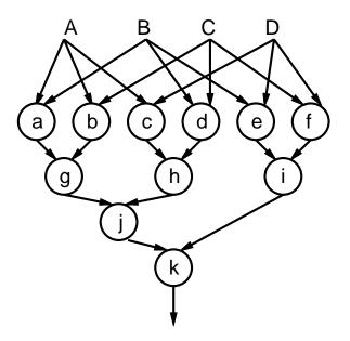
Provide two schedules of the graph onto a set of 2 Functional Units. Both should minimize the schedule length. A, B, C, D start as live state (so the minimum storage required is 4 memory locations); each of these initial 4 memory locations can be reused when the input is no longer needed (*i.e.*, is no longer live). As part of your schedule, list the set of variables which are live following each time step.
