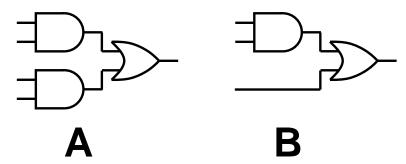
1. If the delay of each gate is 1, what is the delay of each of the circuits?
