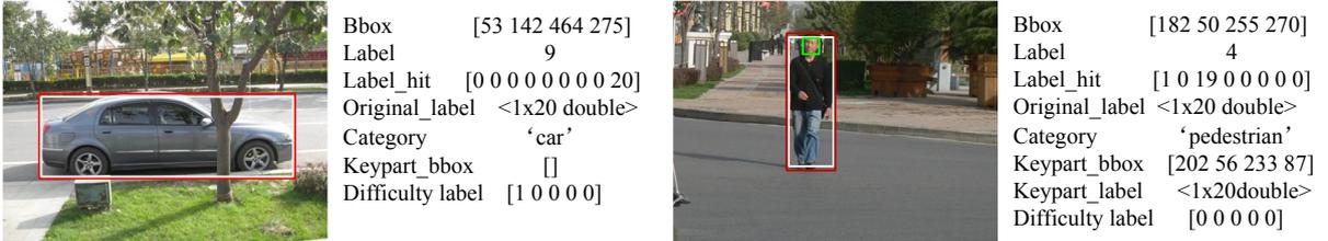
**Figure 3-7** Examples of the final annotation information provided for each object. The “Label\_hit” stands for the transferred votes for each semantic label in the tree structure in a depth first order including the key part clearness label, while the “Label” is the index of the final label after annotation integration. “Original\_label” and “Keypart\_label” are the original labels from the 20 subjects.
