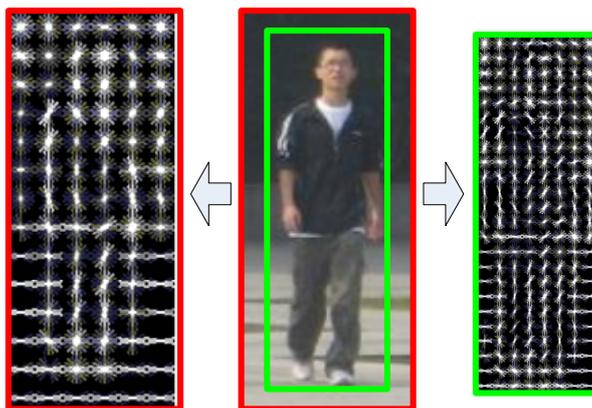
**Figure 4-4** Two-layer HOG features. The coarse scale feature captures big structures of the objects and takes the close context into account, while the fine scale one focuses more on the details of object parts and shape subtleties of the objects themselves.
