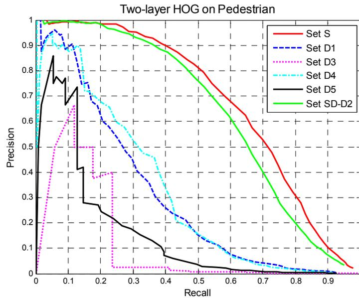
**Figure 3-11** The disorder of the PR curves due to different numbers of positive examples in the listed testing subsets. Since the precision is computed by the true positives vs. true positives plus the false positives, for a given FPPI of the model, it’s more likely that those subsets with more positives have more true positives (i.e., higher precision).
