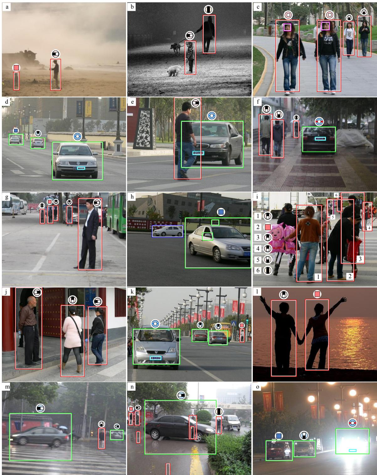
**Figure 4-13** Some representative results of our DLR algorithm on the IAIR-CarPed dataset. The first 4 rows (a-l) are generated by the model trained on set A, while the results in the last row (m-o) are from the model trained on set B. Green and red bounding boxes represent car and pedestrian hypotheses respectively, while blue bounding boxes show the missed ones. The white box within each object bounding box is for contrasting. Semantic signs are attached close to the hypotheses.
