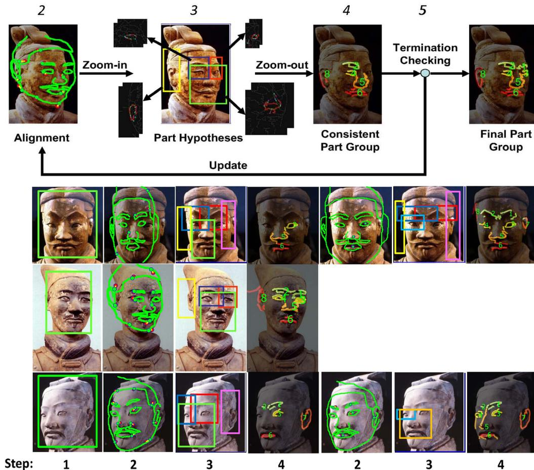
**Figure 5-4** Saliency based opportunistic search, using faces as an example. Top: the flowchart. Bottom: results of each step for 3 different examples. Typically the iteration converges after only one or two rounds. Rectangles with different colors indicate the zoom-in search zones for different parts. Note that when zoom-in is performed for the first time, two adjacent parts can be searched together for efficiency. This figure is best viewed in color.
