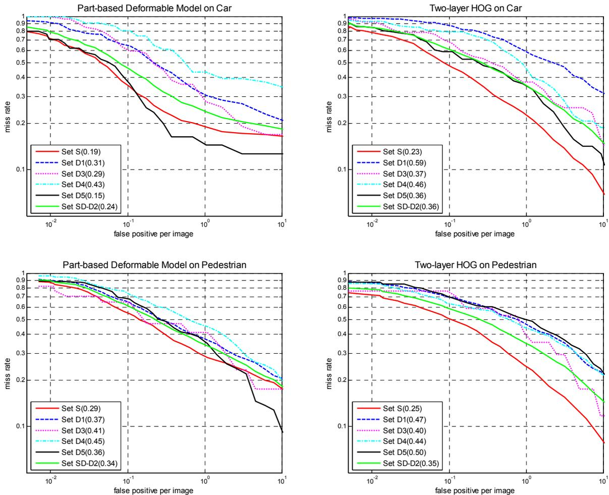
**Figure 3-10** Object detection results measured by per-image DET curves.
