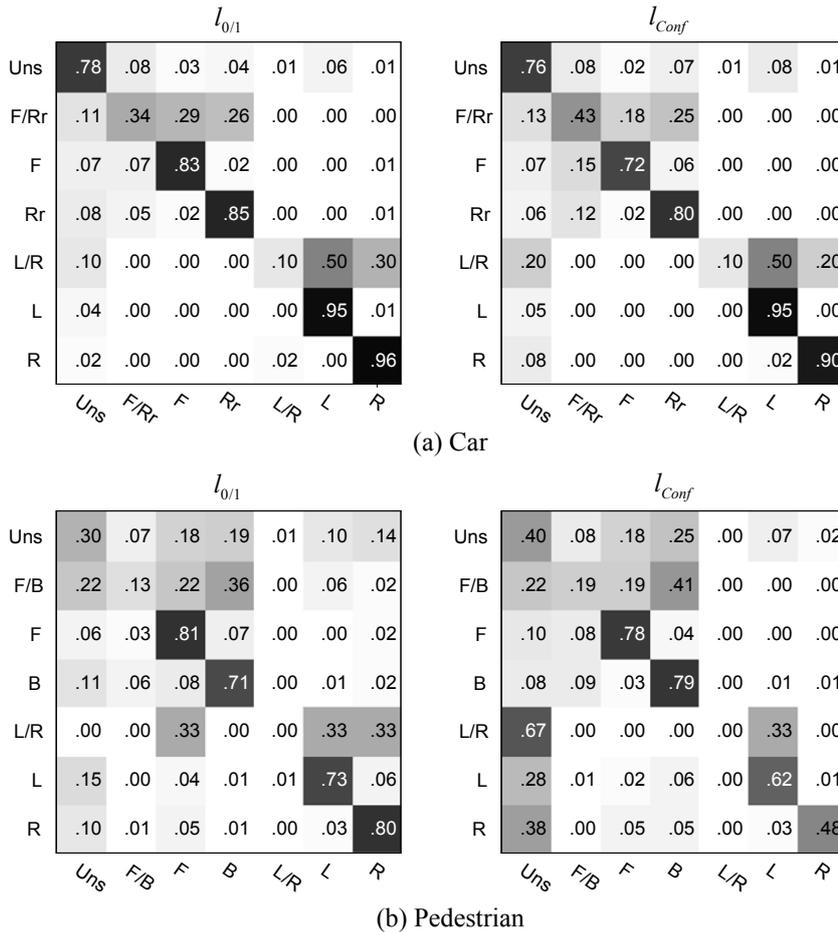
**Figure 3-12** The confusions in the test results using the two different loss functions. It shows that comparing to the flat multiclass classification, structured learning using the relatively more conservative confusion loss can lead to more conservative predictions.
