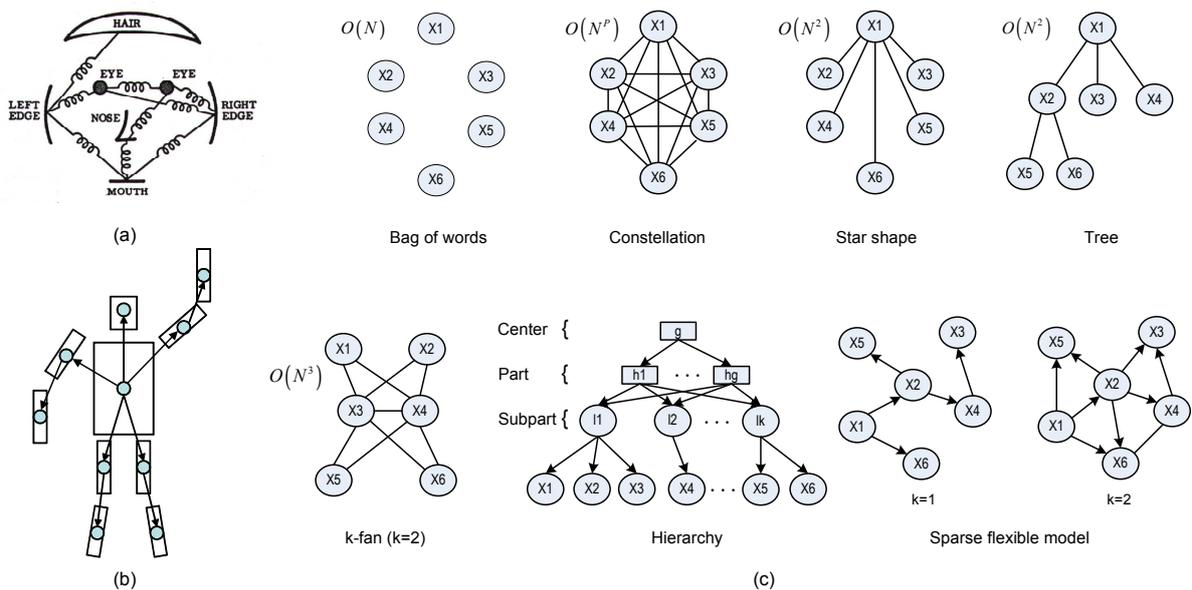
**Figure 2-4** Part-based models: (a) the pictorial structure proposed by Fischler and Elschlager [88]; (b) the commonly used tree structure for human body parsing; (c) some recently proposed structures for part-based models [89]. Note that bag of words model is not a part-based model, and it is presented here only for contrasting.
