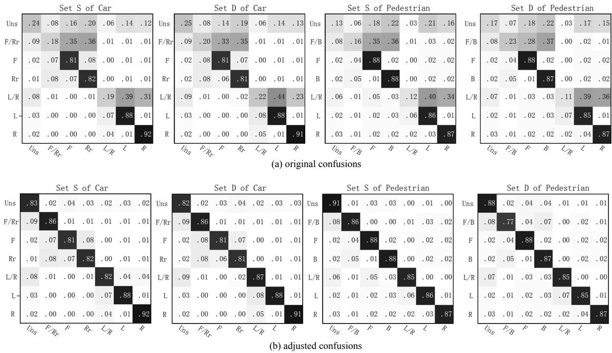
**Figure 3-8** The human confusions on the object orientations through rapid recognition. The upper row shows the human confusions computed using the original labels which are aggressive, while the lower row presents the adjusted confusions which look much more conservative. The adjusted confusions are computed using the transferred labels which significantly prevent predicting ambiguous objects with deeper labels than they should have.
