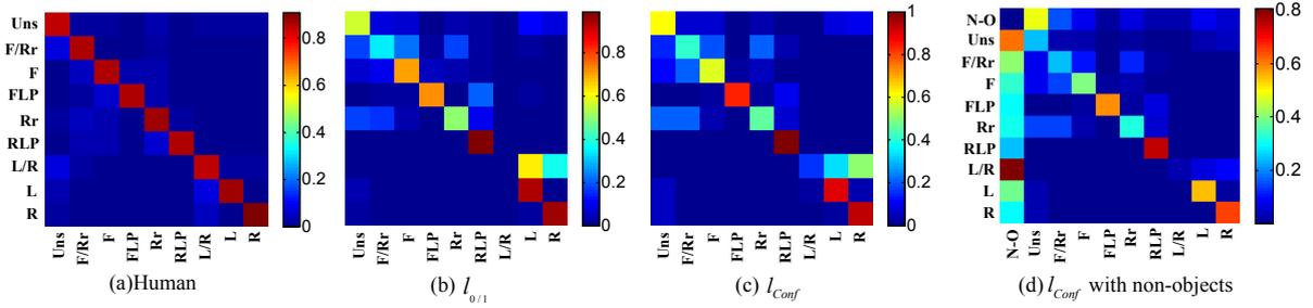
**Figure 4-10** Recognition confusion matrices on set B of “car”. The first three are within-class object categorization confusions of humans, DLR with zero-one loss (i.e. the *multiclass classification*), and DLR with the confusion loss, respectively. The last one is that of DLR with confusion loss on the whole categorization problem including the non-object category (denoted by “N-O”). Each row is normalized to sum to 1.
