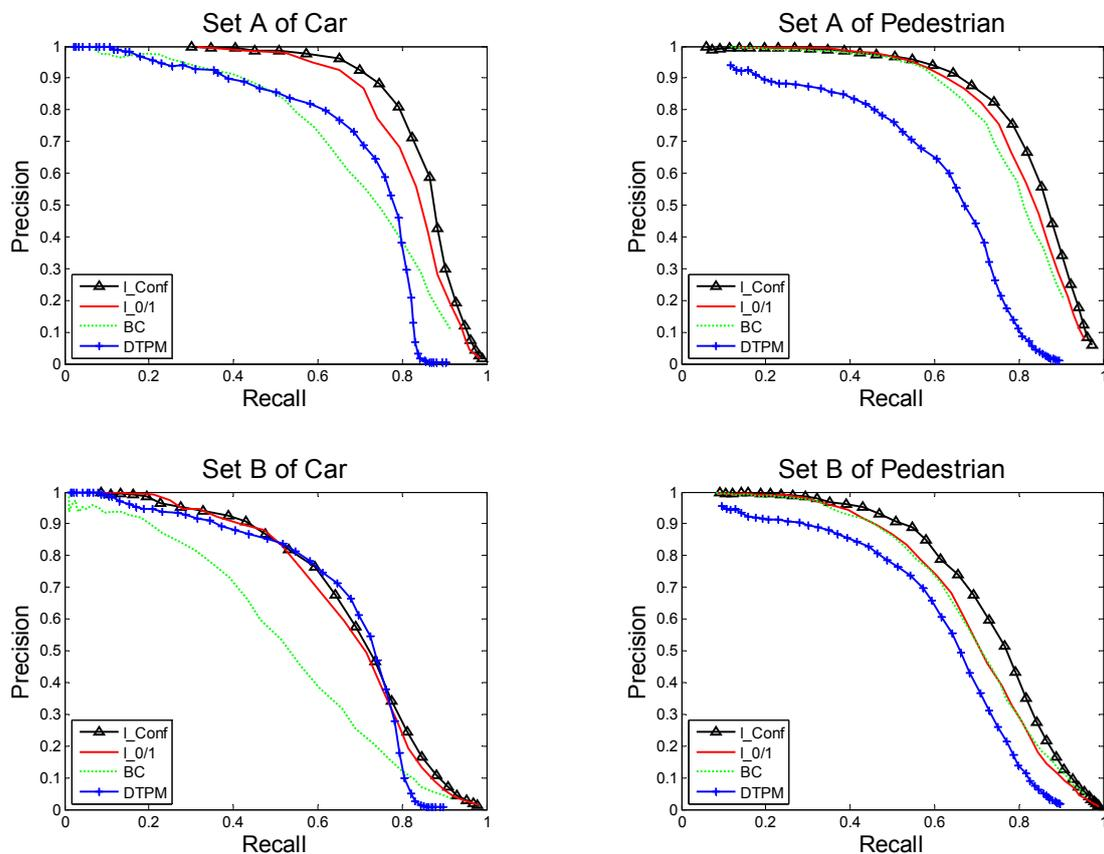
Figure 4-9 Precision-recall curves on category-level recognition.
