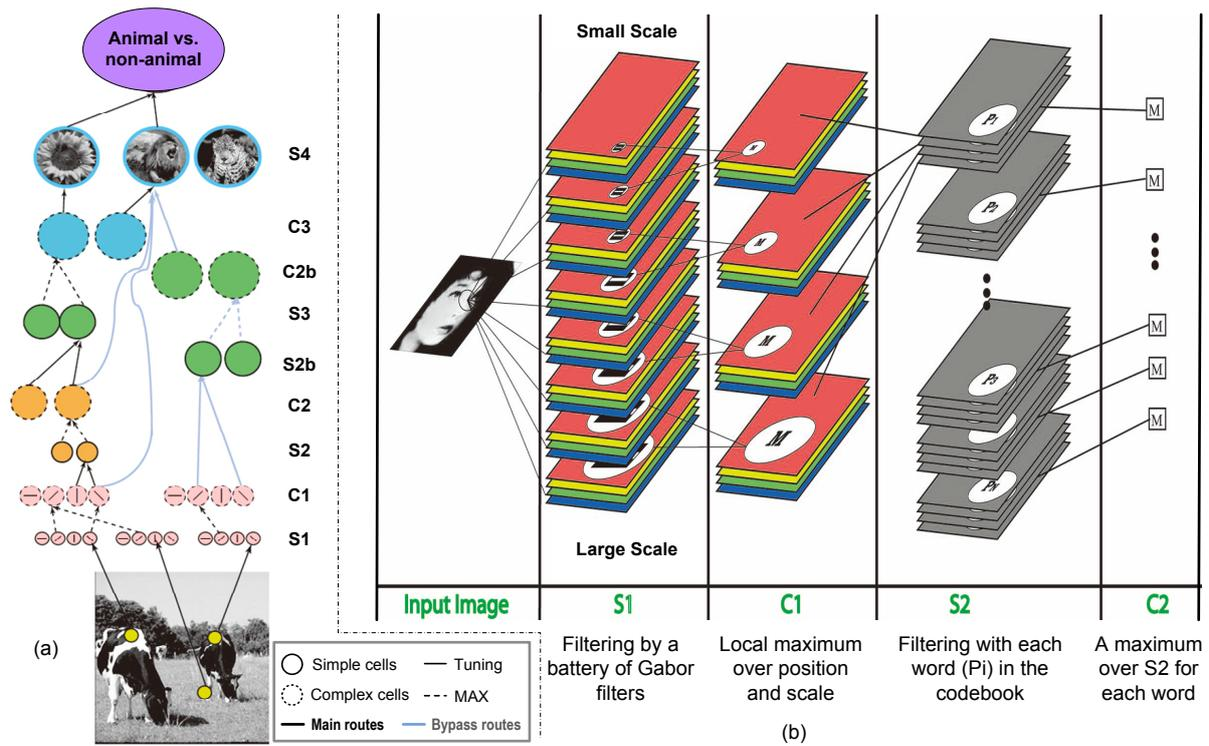
**Figure 2-5** A biologically inspired feedforward recognition model: (a) the functional primitives of the feedforward model<sup>[5]</sup>; (b) the feedforward computational model<sup>[4]</sup>. Due to the space, only 8 of the 16 scales at S1 are shown. “M” stands for the MAX operation, while “P” denotes a word in the codebook (in the original model it is just an image patch).
