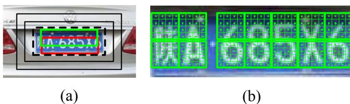
**Figure 4-6** Features for training the license plate detector: a) regions for extracting statistical gradient features and b) an example of the extracted SIFT features.
