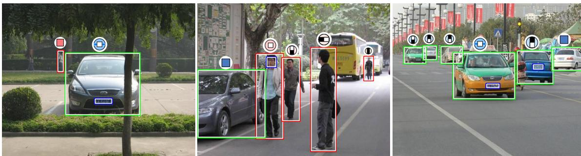
**Figure 3-3** Example images and their annotations. Green and red bounding boxes represent annotated cars and pedestrians respectively, while the sign above each object illustrates its semantic label.
