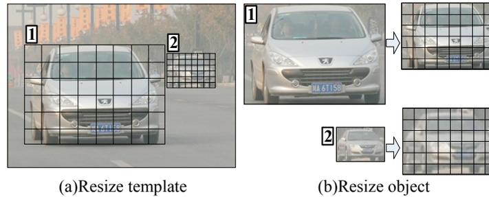
**Figure 4-3** Scale-sensitive subpixel features. Instead of resizing the object to fit a fixed feature template like (b), we resize the template to fit the data as shown in (a). The subpixel-level feature descriptor represents the subtle differences of objects with different scales.
