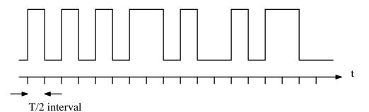
(b) Now assume that the waveform represents differential Manchester coding, and find the two possible bit streams.
