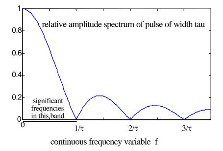
From this we may conclude that the highest frequency we need in the representation of a single rectangular pulse of width  $\tau$  is approximately  $\frac{1}{t}$ , because roughly speaking the significant frequencies are those below this limit (the others have relatively low amplitudes).
