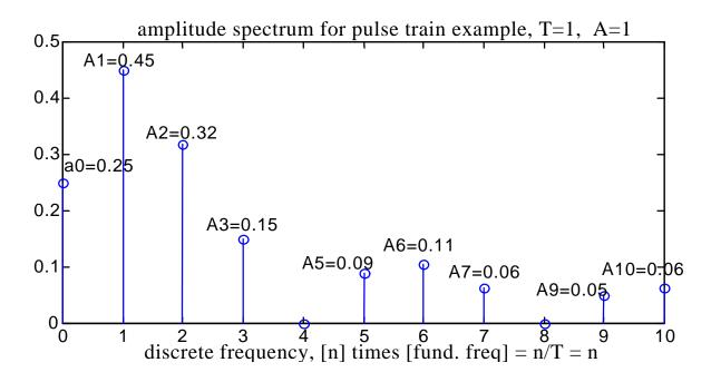
Such a plot helps us decide the highest frequency that we need for a good approximation to the original periodic function, in this case for the pulse train. From the plot above we may decide that beyond frequency 4 Hz, none of the Fourier coefficients have significant magnitude and may be neglected.
