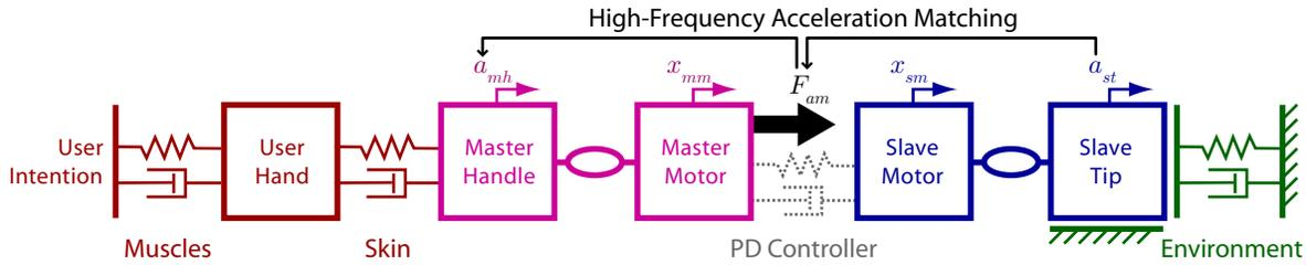
Fig. 4. In the proposed approach, an additional force,  $F_{am}$ , matches the high-frequency accelerations of the master handle,  $\tilde{a}_{mh}$ , to those of the slave tip,  $\tilde{a}_{st}$ , while a standard PD controller provides the user with low-frequency haptic feedback.
