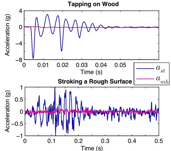
Fig. 3. Slave tip and master handle accelerations,  $a_{st}$  and  $a_{mh}$  respectively, do not match when tapping on a piece of wood or stroking a roughly textured object under bilateral proportional-derivative control.
