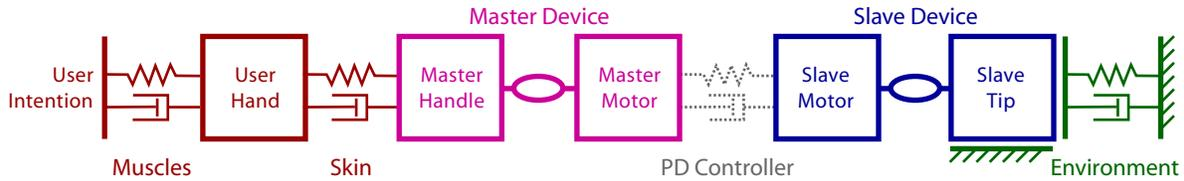
Fig. 2. A lumped parameter model of a telerobotic system under bilateral PD control. The user’s influence on the system is approximated as a position set-point attached to the master handle through the arm muscles, hand, and skin. For clarity, only one member is depicted between the endpoint and motor of both master and slave mechanisms, though these connections can include several spring-like, dissipative, and inertial elements.
