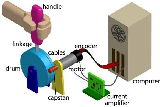
Fig. 2. The master’s long dynamic chain connects the user to the controller.
