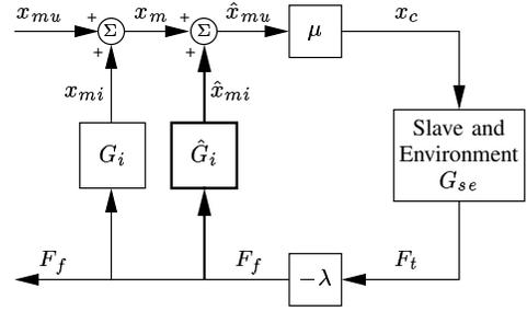
Fig. 7. Induced master motion can be canceled using the model  $\hat{G}_i$ .
