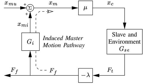
Fig. 5. Motion induced by the force feedback,  $x_{mi}$ , superimposes with motion intended by the user,  $x_{mu}$ , at the master motor. The passive dynamics of the user-master system,  $G_i$ , govern the pathway of induced master motion.
