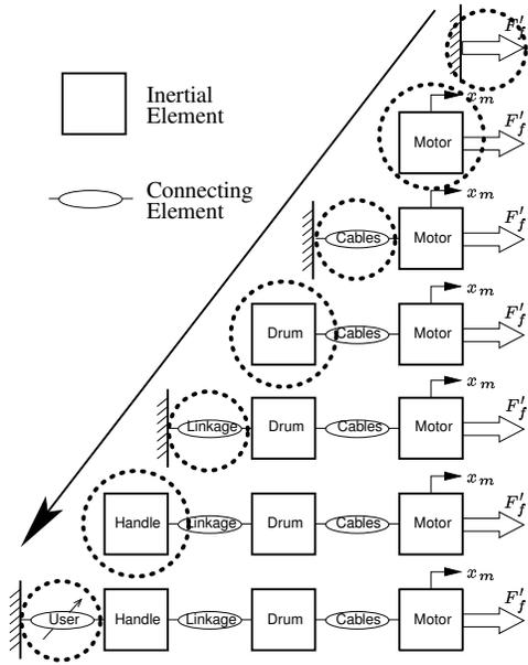
Fig. 8. Successive isolation of the user-master system progresses from the force command through the motor, cables, drum, linkage, handle, and user.
