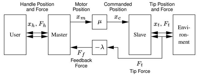
Fig. 3. In position-force control, the slave is commanded to track the master’s position, and the master mechanism recreates tip interaction forces for the user.
