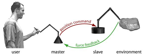
Fig. 1. A telerobotic system connects the user to the environment via master and slave robots.
