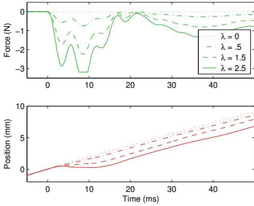
Fig. 4. Display of a scaled, pre-recorded force profile to a user executing a constant motion. Increasing the force scale  $\lambda$  generates motor movement that is not intended by the user.
