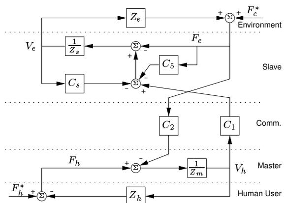
Fig. 14. Cancellation of induced master motion is implemented via  $C_5$  in the general architecture for teleoperation.
