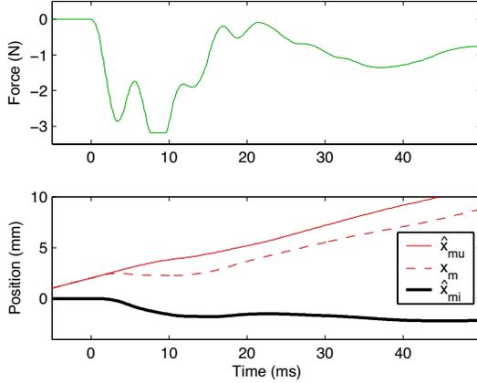
Fig. 12. The full model accurately predicts induced master motion during open-loop display of a pre-recorded force profile, providing a smooth estimate of user intention,  $\hat{x}_{mu}$
