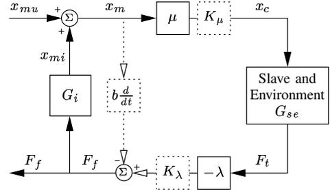
Fig. 6. Position-force control with three compensation options: local derivative feedback on master position via  $b \frac{d}{dt}$ , position command filter  $K_\mu$ , and force feedback filter  $K_\lambda$ .
