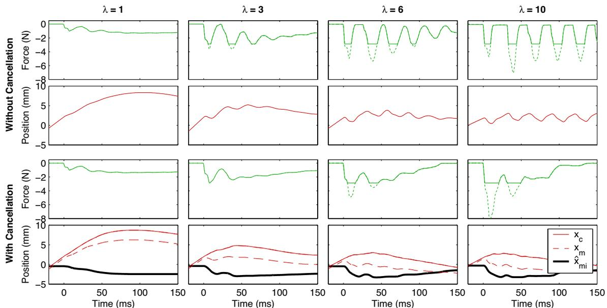
Fig. 13. Force feedback,  $F_f$ , and slave position command,  $x_c$ , with and without cancellation for a range of  $\lambda$  values, keeping  $\mu = 1$ . Contacts are stabilized by canceling induced master motion from the measured master position,  $x_m$ , using the model's real-time estimate,  $\hat{x}_{mi}$ .
