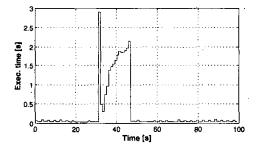
Figure 3: Execution time measurement for the MPC algorithm in the specific simulation scenario given by Figure 2.
