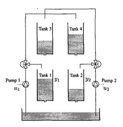
Figure 1: The quadruple-tank laboratory process. From [9].
