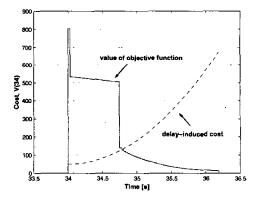
Figure 4: The solid curve shows a close-up of how the objective function (1) decreases for each iteration during a sample when the execution time is long. It is seen that the required execution time for full optimization is well above the period of one second.
