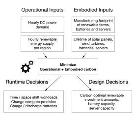
Figure 4: A framework for carbon-free datacenter design.
