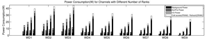
Figure 8: Power as rank count increases. As in Figure 7, for each workload, bars show nRank(PCM) followed by nRank(DRAM),  $n \in [4, 8, 16, 32]$ .
