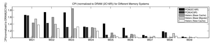
Figure 10: Application delay (cycles per instruction) for alternative memory architectures. Bars show instructions per cycle normalized to homogeneous DRAM(2C16R).
