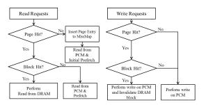
Figure 6: Management for fine-grained DRAM cache. Flow implemented by master controller.
