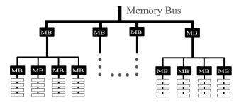
Figure 4: Buffering with hierarchical topology. With 20 buffers (black), 64 memory ranks (white) share a memory bus to the slave.
