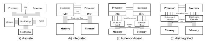
Figure 1: Memory controller architectures.
