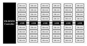
Figure 3: Buffering with Fully-Buffered DIMMs (FB-DIMM)
