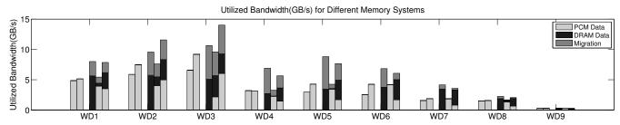
Figure 11: Sustained bandwidth for alternative memory architectures. Bars show PCM (2C16R), PCM (4C8R), Hetero (Base Cache), Hetero (Base Migrate), Hetero (New Cache).
