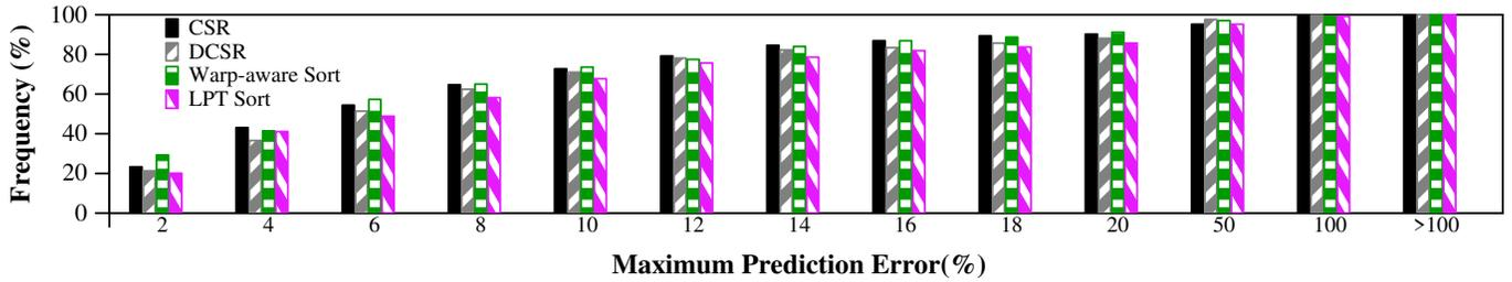
Fig. 12: Cumulative distribution of absolute errors on predicted execution time for each of the 4 classes. 70% of our predictions report errors below 10%.
