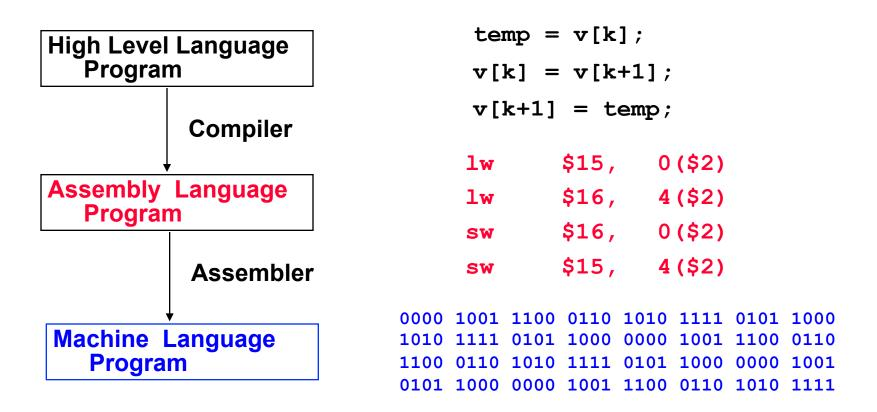
Assembler program automatically converts assembly code into the binary machine language (zeros and ones) that the computer actually executes
