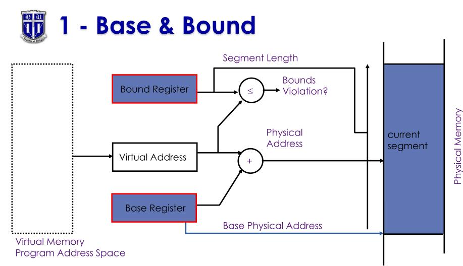
Base register – Identifies a program's allocation in physical memory. Bound register – Provides protection and isolation between programs Base, Bound registers visible only when processor is running in "supervisor" mode
