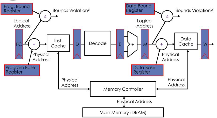
Every access to memory requires translating virtual addresses to physical addresses. Efficient adder implementations are possible for (base+offset). • ECE 252 / CPS 220
