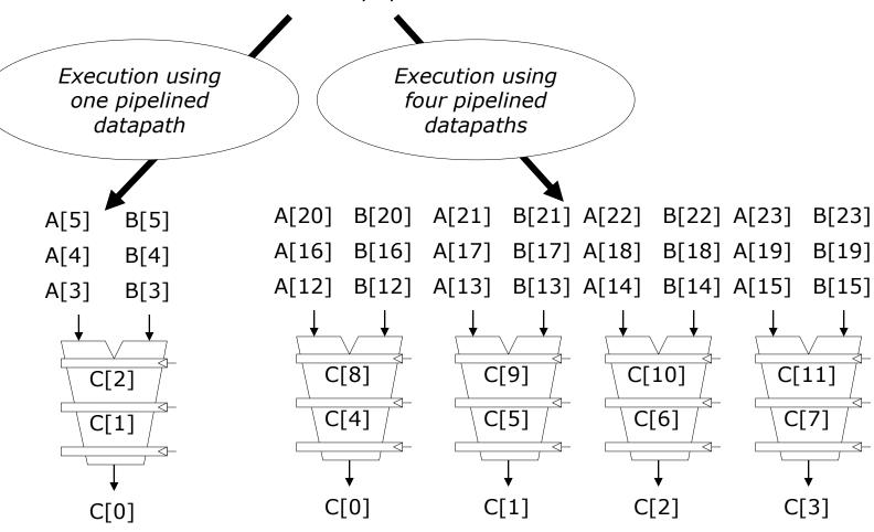
1 adder → 1 element / cycle N cycles
