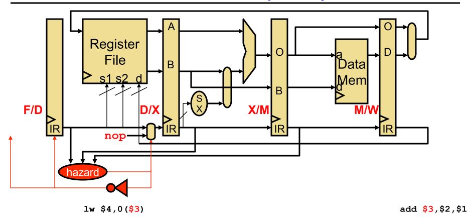
(F/D.IR.RS1 == D/X.IR.RD) || (F/D.IR.RS2 == D/X.IR.RD) || (F/D.IR.RS1 == X/M.IR.RD) || (F/D.IR.RS2 == X/M.IR.RD) = **0**
