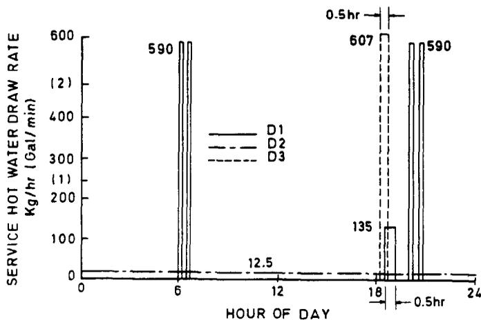
Fig. 6. Daily draw pattern of domestic hot water:  $D_1$  = characteristic national;  $D_2$  = uniform;  $D_3$  = lumped at the end of the day. The duration of each of the 590 kg/hr draws is 0.1 hr.
