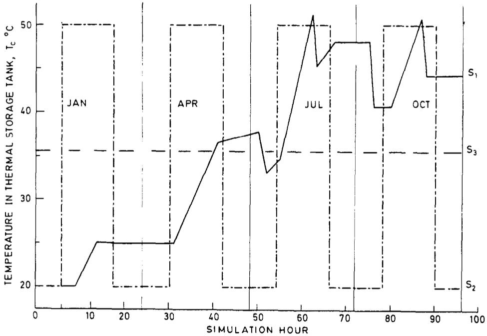
Fig. 5: Variation patterns of the solar-collector-heated thermal storage water temperature:  $S_1$  = computed pattern for SolaRow;  $S_2$  = square wave pattern;  $S_3$  = constant continuous draw.
