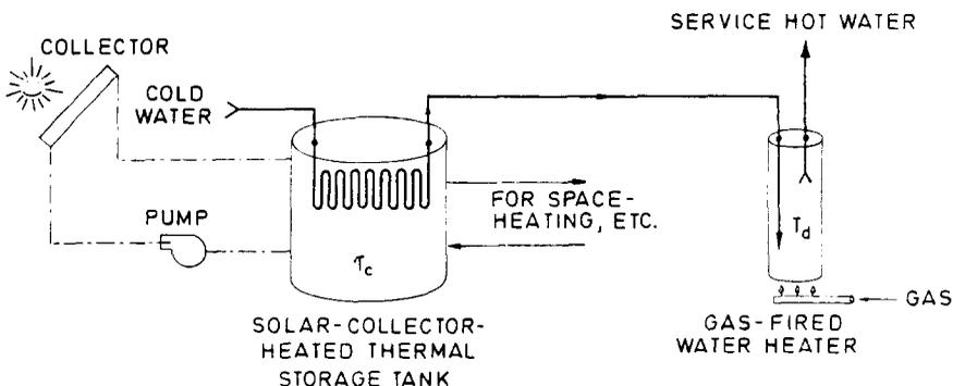
Fig. 2. Flow diagram of the straight-through system.
