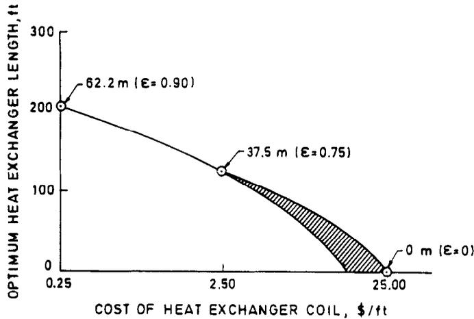
Fig. 4. Optimal length of the heat-exchanger coil.
