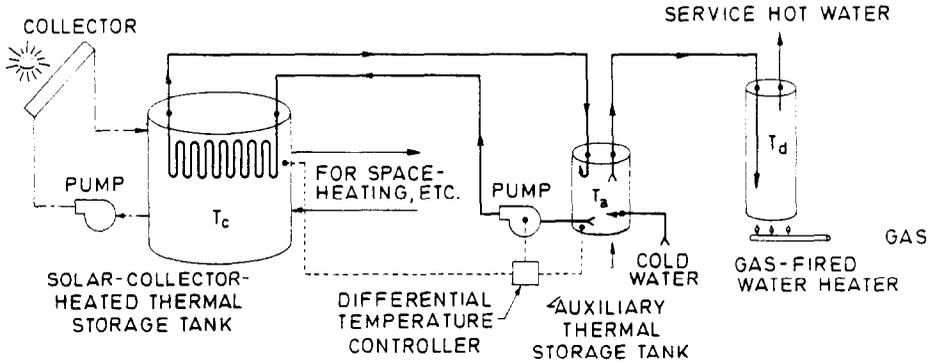
Fig. 1. Flow diagram of recirculation system.
