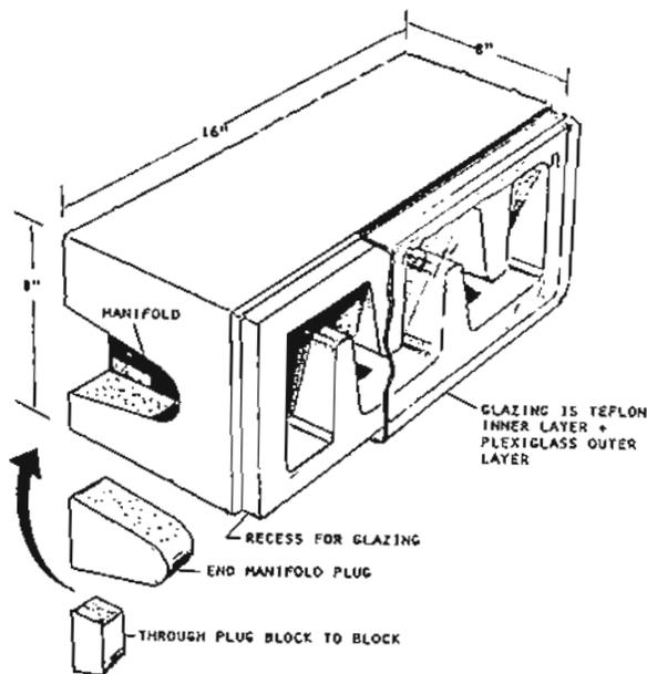
a. The standard size (8" × 8" × 16") air-heating concrete block
