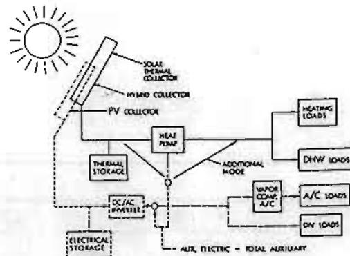
(c) Series Heat Pump Hybrid Solar Power System
