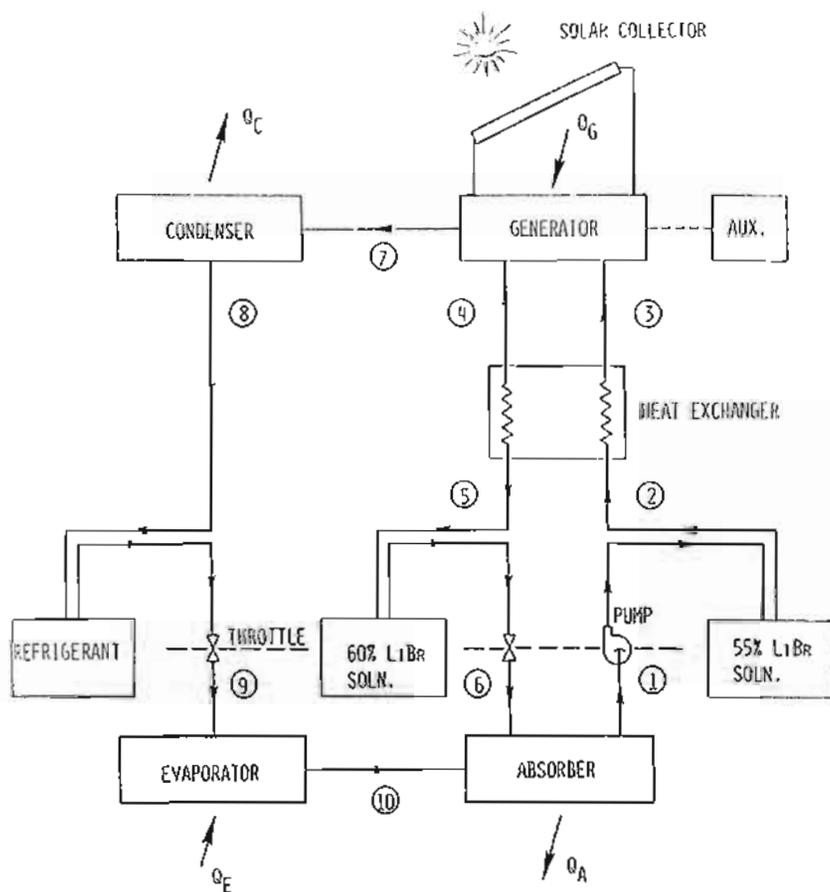
Figure 17.8 Schematic of solar-assisted absorption heat pump with integral refrigerant and solution storage. Source: Schrenk and Lior (1975).
