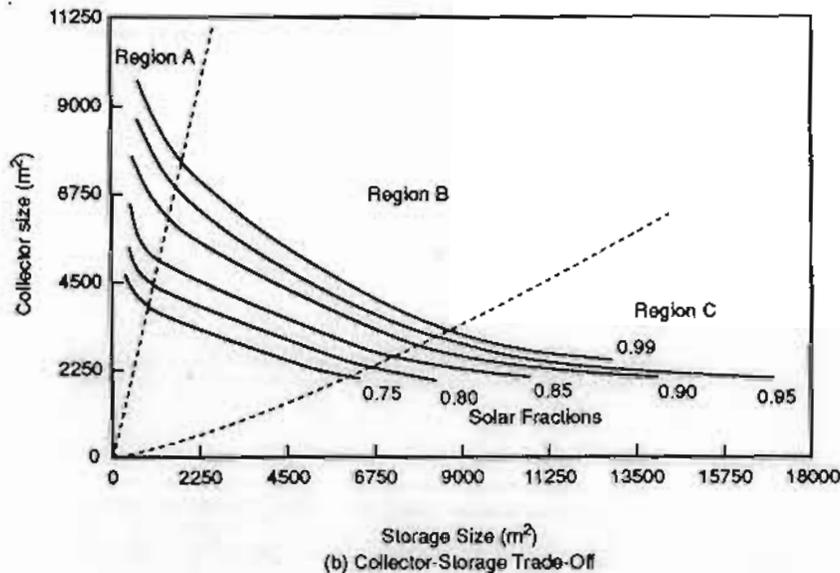
Figure 17.16 System performance and collector storage tradeoff curve for a typical annual storage system. Source: Sillman (1981).
