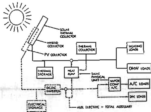
(b) Parallel Heat Pump Hybrid Solar Power System
