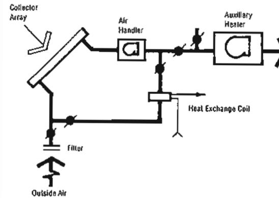
This system combines outside air and water heating. The combined system is often preferable in order to utilize the solar system throughout the year. In cases where hot air demands are intermittent, the system stores energy for hot water requirements.
