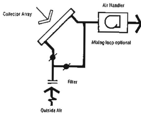
Heating outside air is often the simplest, most cost-effective use of the Solaron system. Outside air is drawn or blown through the collector array where the air is heated. BTU delivery is maximized in this system since the inlet air is at ambient temperature, thereby reducing losses from the collectors.
