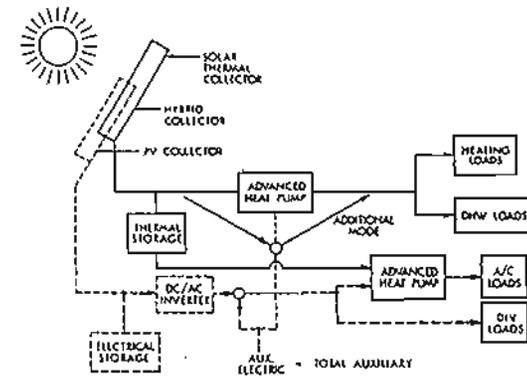
(e) Series Advanced Heat Pump Hybrid Solar Power System
