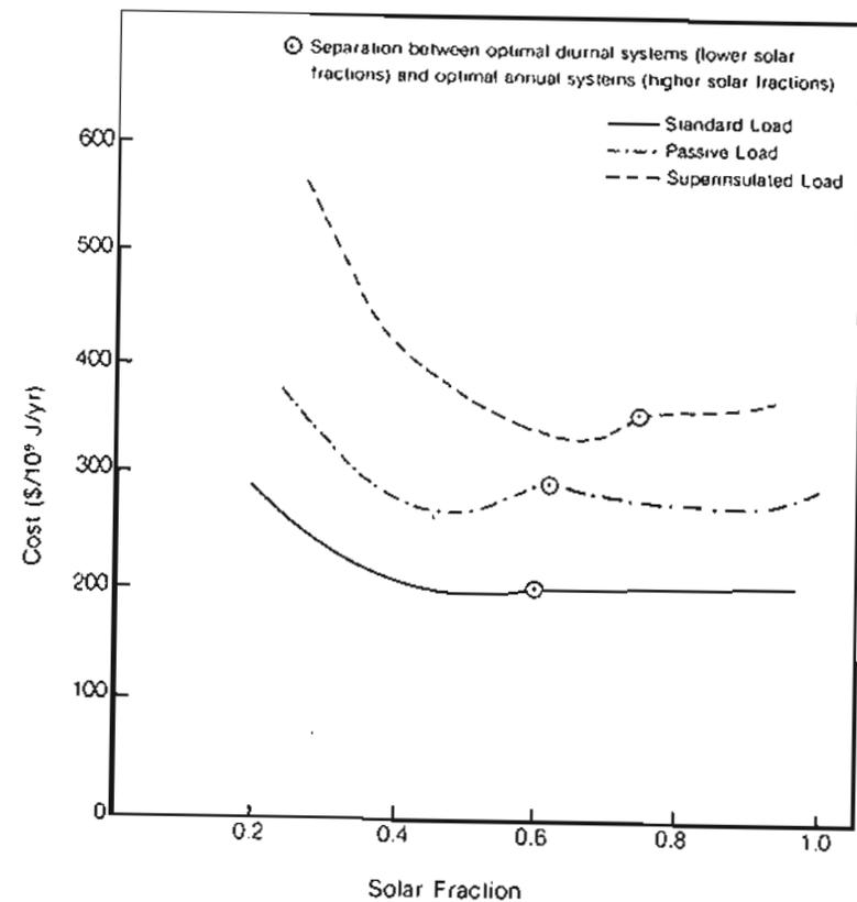
Figure 17.17 System cost per unit heat delivered vs. solar fraction for combined space heat and hot water systems. Source: Sillman (1981).
