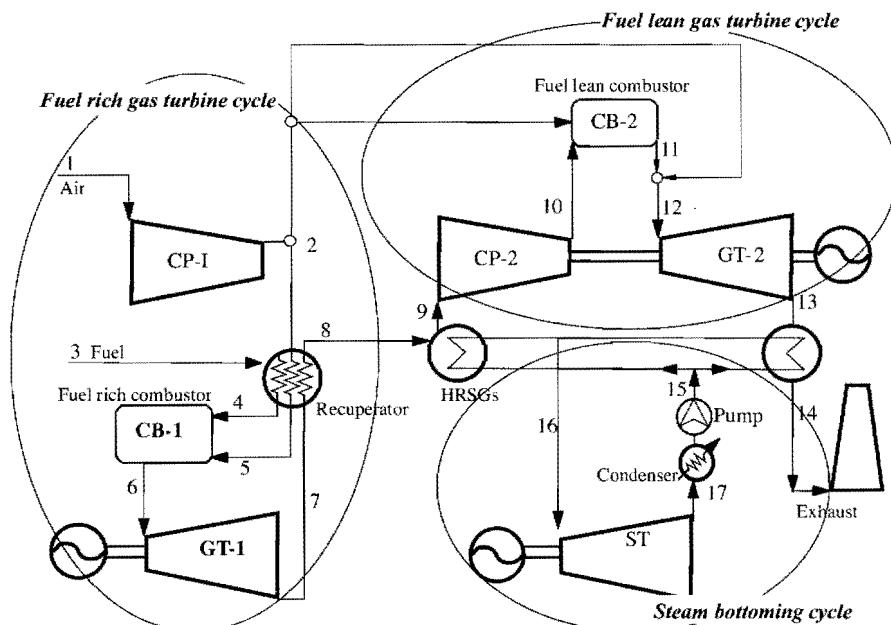
Fig. 1 Flow diagram of the combined cycle based on the ChGT.
