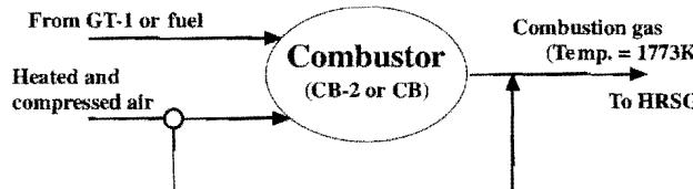
**Fig. 3** Flow detail for the ChGT (Fig. 1) and for the CB of the conventional combined cycle (Fig. 2).
