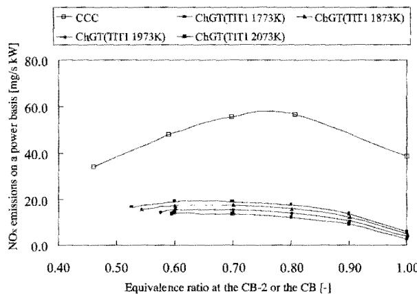
Fig. 8 NO<sub>x</sub> emissions of the ChGT system in comparison with the CCC.
