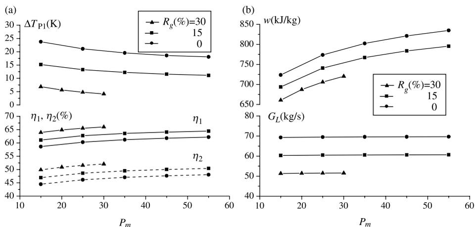
Fig. 7. The influence of  $P_m$  and  $R_g$  ( $t_6=1300\text{ }^\circ\text{C}$ ,  $P_h=150\text{ bar}$ ).
