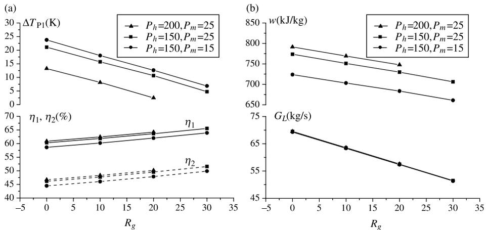
Fig. 6. The influence of  $P_h$ ,  $P_m$  and  $R_g$  ( $t_6=1300$  °C).
