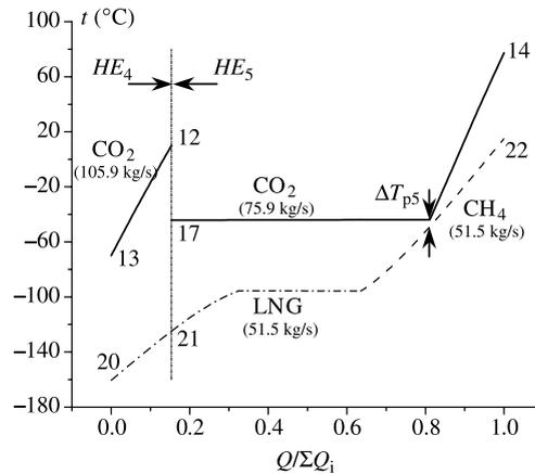
Fig. 4.  $t$ - $Q$  diagram in the LNG evaporation system.
