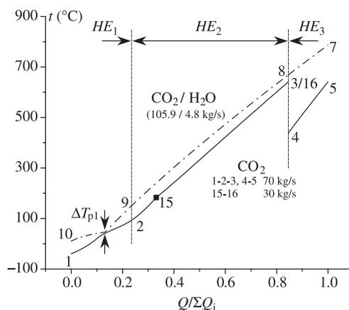
Fig. 3.  $t$ - $Q$  diagram in the CO<sub>2</sub> recuperation system.
