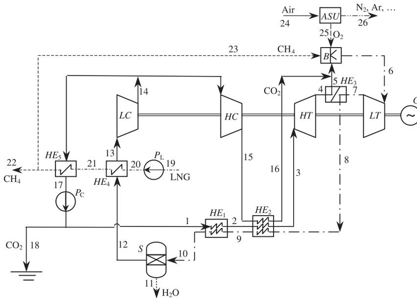
ASU – Air separation unit B – Combustor G – Generator HE – heat exchanger
