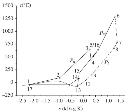
Fig. 2.  $t$ - $s$  diagram for CO<sub>2</sub> cycle.
