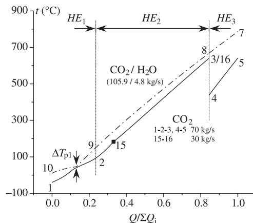
Fig. 3.  $t-Q$  diagram in the CO<sub>2</sub> recuperation system.
