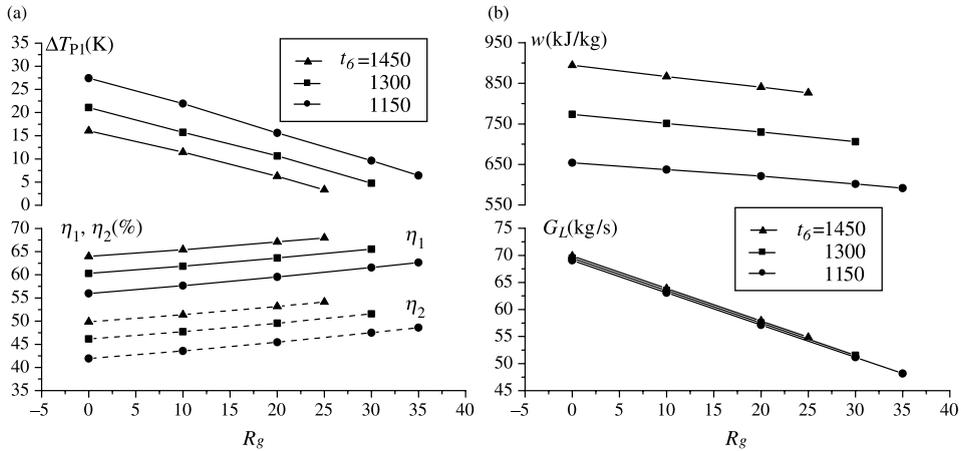
Fig. 5. The influence of  $t_6$  and  $R_g$  ( $P_h=150$  bar,  $P_m=25$  bar).
