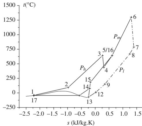
Fig. 2. *t-s* diagram for CO<sub>2</sub> cycle.
