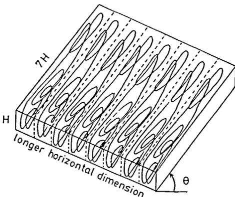
FIG. 1. Sketch of roll cells in an inclined enclosure.
