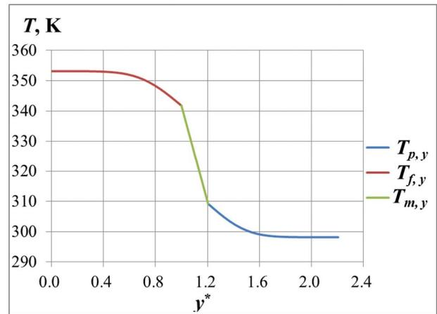
Fig. 16. The temperature as a function of  $y^*$  at fixed  $x^* = 50$  for  $T_{f,i} = 353.15$  K.
