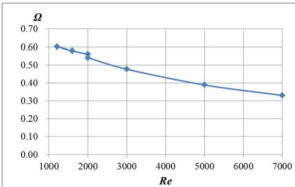
Fig. 20. The relative heat transfer resistance ( $\Omega$ ) as a function of  $Re$  (laminar and turbulent).
