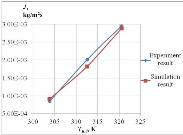
Fig. 8. The computed mass flux for different feed inlet temperature in this study, compared with experimental results from [43]. ( $T_{p,i} = 14^\circ\text{C}$ ,  $u_{f,i} = 0.0635\text{ m/s}$ ,  $u_{p,i} = 0.0635\text{ m/s}$ ,  $l_{ch} = 0.055\text{ m}$ ,  $h_{ch} = 0.002\text{ m}$ ,  $\delta = 125\ \mu\text{m}$ ,  $d_p = 0.32\ \mu\text{m}$ ,  $\epsilon = 0.75$ ,  $\chi = 1.7$ ,  $k_s = 0.22\text{ W/(m}\cdot\text{K)}$ ).
