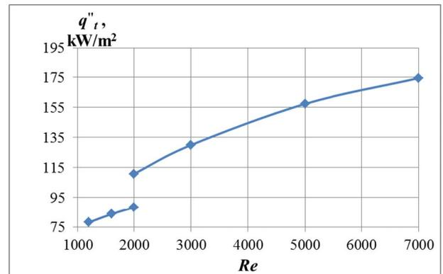
Fig. 23. The total heat flux ( $q_t$ ) as a function of  $Re$  (laminar and turbulent).
