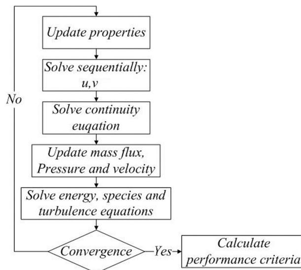
Fig. 6. Logic flow of the solution in Fluent.
