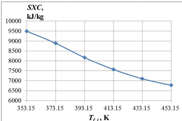
Fig. 14. The specific exergy consumption (SXC) as a function of  $T_{f,i}$ .
