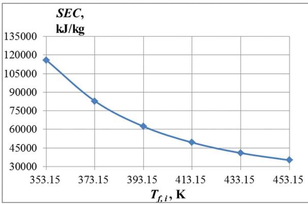
Fig. 13. The specific energy consumption (SEC) as a function of  $T_{f,i}$ .
