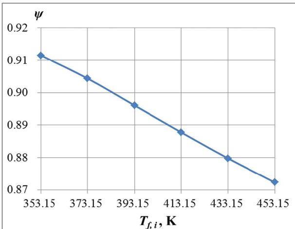
Fig. 15. The exergy efficiency ( $\psi$ ) as a function of  $T_{f,i}$ .
