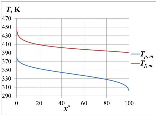
Fig. 19. The  $T_{f,m}$  and along membrane/feed interface ( $y^* = 1^+$ ) and  $T_{p,m}$  along membrane/permeate interface ( $y^* = 1^-$ ) for  $T_{fi} = 453.15$  K.
