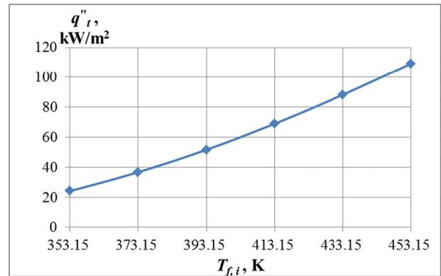
Fig. 12. The total heat flux ( $q_t''$ ) as a function of  $T_{f,i}$ .
