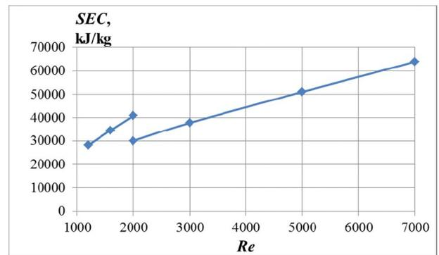
Fig. 24. The specific energy consumption ( $SEC$ ) as a function of  $Re$  (laminar and turbulent).
