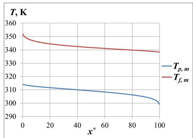
Fig. 18. The  $T_{f,m}$  and along membrane/feed interface ( $y^* = 1^+$ ) and  $T_{p,m}$  along membrane/permeate interface ( $y^* = 1^-$ ) for  $T_{f,i} = 353.15$  K.
