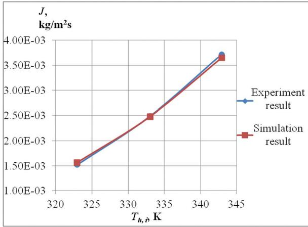
Fig. 7. The computed mass flux for different feed inlet temperature in this study, compared with experimental results from [42]. ( $T_{p,i} = 20^\circ\text{C}$ ,  $u_{f,i} = 0.0632\text{ m/s}$ ,  $u_{p,i} = 0.0632\text{ m/s}$ ,  $l_{ch} = 0.1\text{ m}$ ,  $h_{ch} = 0.004545\text{ m}$ ,  $\delta = 126\ \mu\text{m}$ ,  $d_p = 0.22\ \mu\text{m}$ ,  $\epsilon = 0.62$ ,  $\chi = 2$ ,  $k_s = 0.041\text{ W/(m}\cdot\text{K)}$ ).
