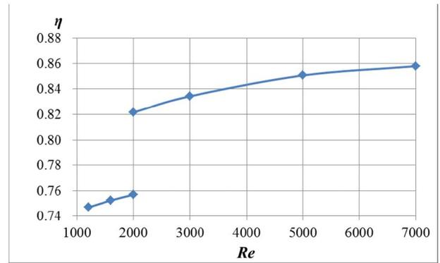
Fig. 22. The membrane thermal efficiency ( $\eta$ ) as a function of  $Re$  (laminar and turbulent).
