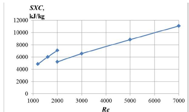
Fig. 25. The specific exergy consumption ( $SXC$ ) as a function of  $Re$  (laminar and turbulent).
