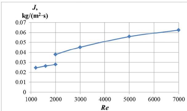
Fig. 21. The mass flux ( $J$ ) as a function of  $Re$  (laminar and turbulent).
