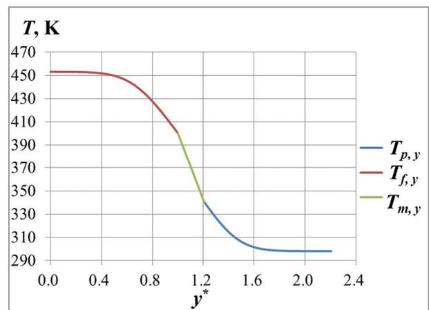
Fig. 17. The temperature as a function of  $y^*$  at fixed  $x^* = 50$  for  $T_{f,i} = 453.15$  K.
