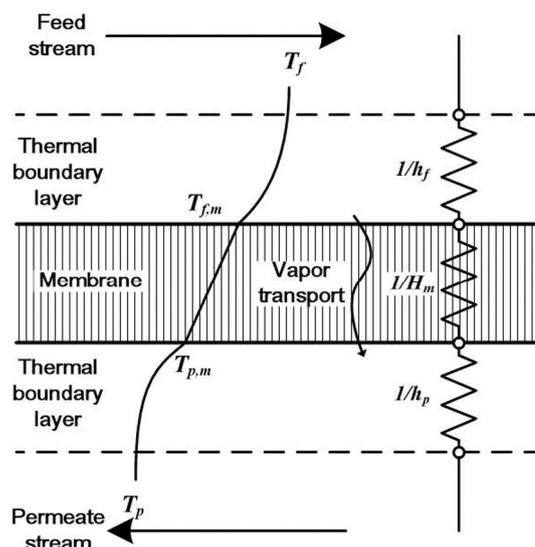
Fig. 2. Qualitative depiction of the temperature profile, vapor mass transport, and heat transfer resistance analog in DCMD.
