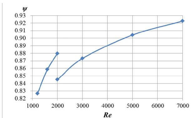
Fig. 26. The exergy efficiency ( $\psi$ ) as a function of  $Re$  (laminar and turbulent).
