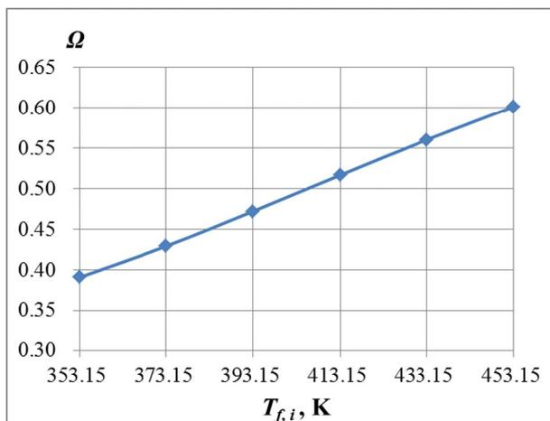
Fig. 9. The relative heat transfer resistance ( $\Omega$ ) as a function of  $T_{f,i}$ .
