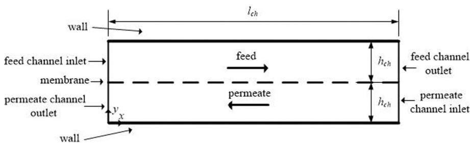
Fig. 1. Schematic of the studied DCMD module.
