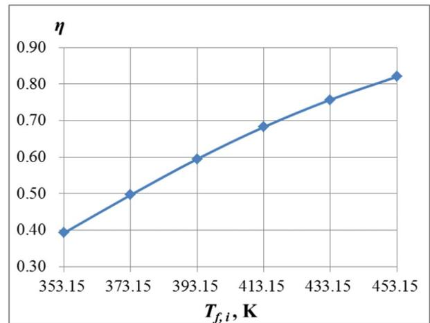
Fig. 11. The membrane thermal efficiency ( $\eta$ ) as a function of  $T_{f,i}$ .
