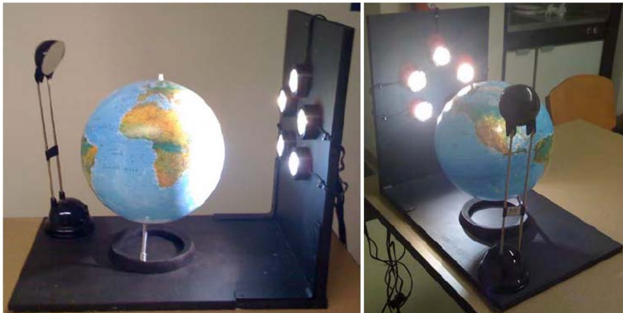
Fig. 4: Simplified concept demonstration model of a Sun-Earth orbital mirror system showing light on one side of earth (left image) and reflected light on the dark side of earth (right image). Built by the author’s students Betsy Rosenblatt, Travis Schlegel and Kamal Shair, 2008.
